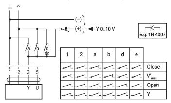
Override control and limiting with DC 24 V with relay contacts
