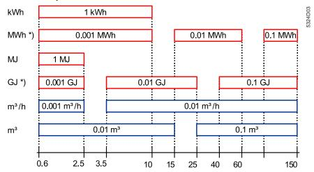
\*) Decimal places "flashing", "static", or "suppressed"
